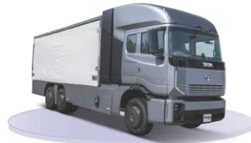
Prima H.28 Indigenously developed H2 ICE truck with a range of ~550 km
